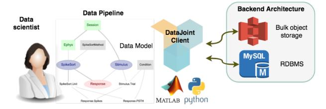
Fig. 3: Conceptual overview of DataJoint operation.
